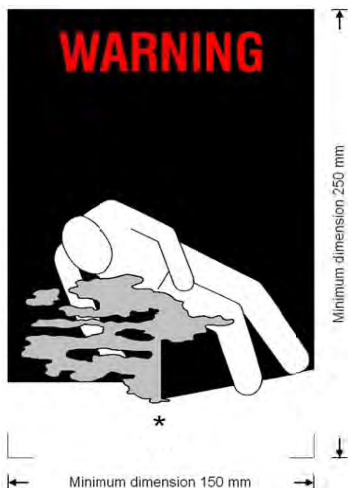
Figure 5.5.2: Asphyxiation warning mark for cargo transport units
