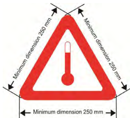
Figure 5.3.4: Mark for carriage at elevated temperature
